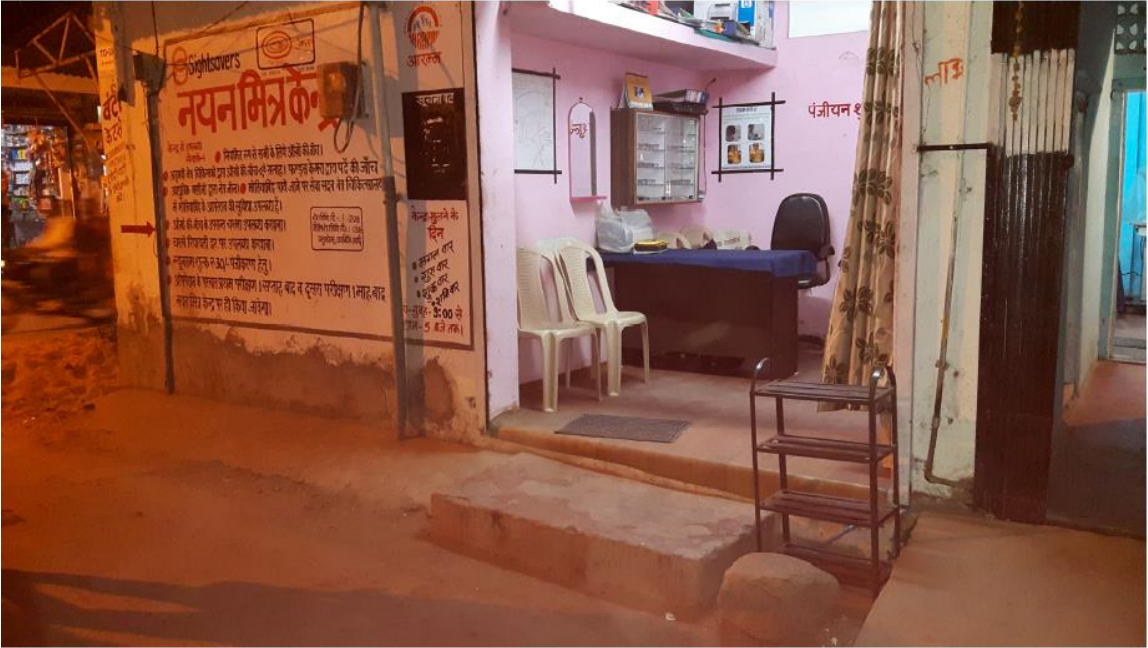
Figure 1. The enquiry counter at CHC Kolar Road vision centre is not accessible, being at a height of 1120 mm, with a communication opening at 1550 mm.
